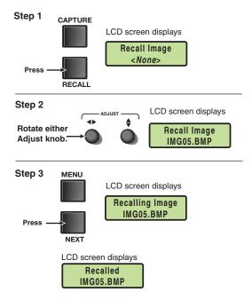
Figure 14. Sequence for Recalling an Image
